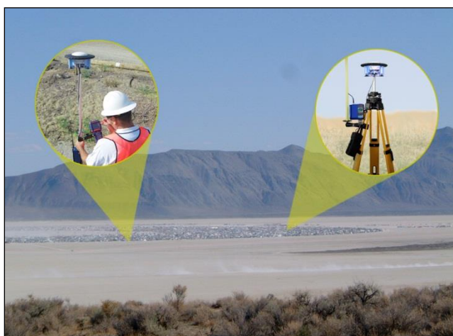
Figure 36: RTK Setup - Good Line of Sight
